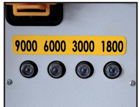
4 vitesses de rotation Spindle moulder with 4 speed
